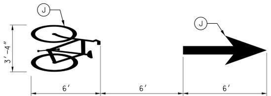
BICYCLE LANE PAVEMENT MARKING DETAIL SCALE: NOT TO SCALE
